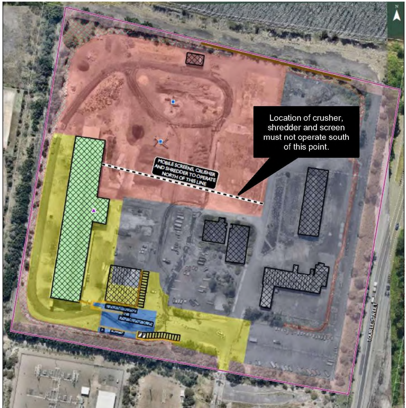
Figure 2-5 Limits on Location of Crusher, Shredder and Screens
