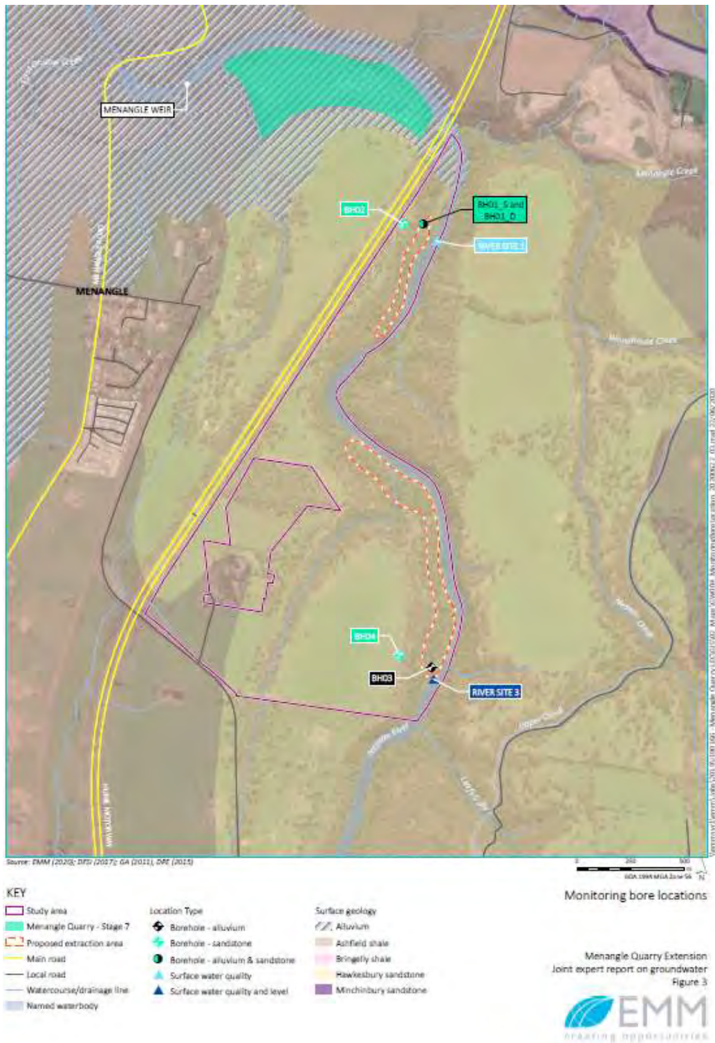
Figure 7 - Groundwater Monitoring Locations
