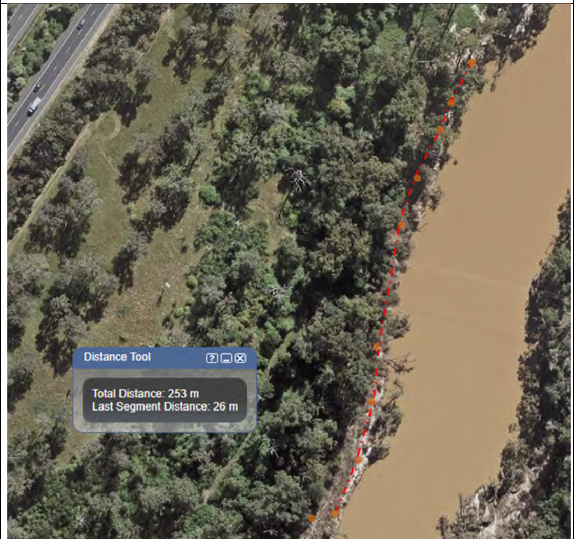
Figure 4-5 Benedict Survey Drawing Stage 8B 10m River Offset Boundary Survey Peg Locations (20 November 2023)
