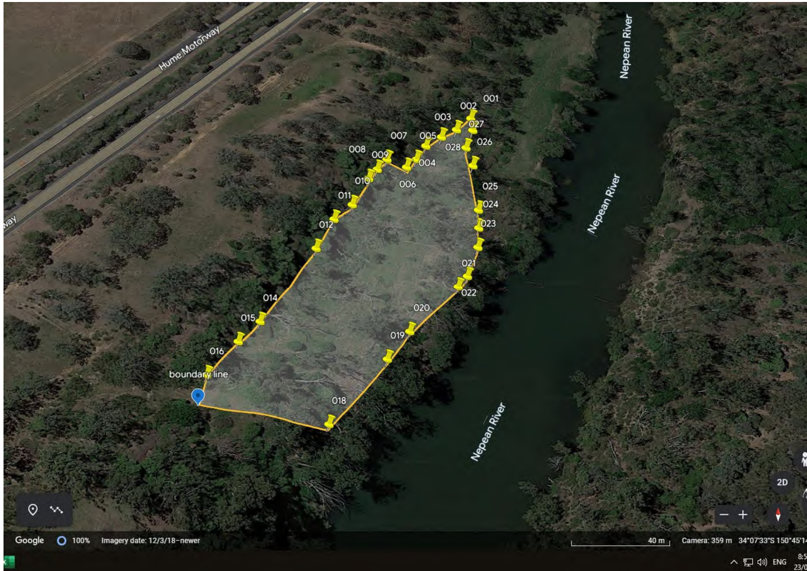
Figure 4-1 Benedict Survey Drawing for Stage 8A Extraction Boundary Survey Peg Locations (23 August 2023)
