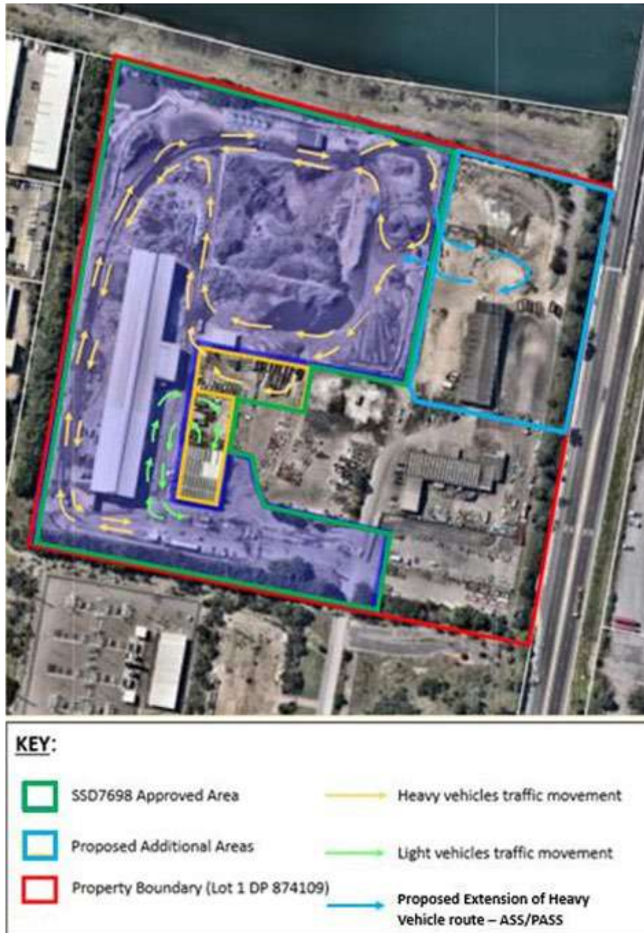
Figure 2.3 Vehicle traffic flow plan (Approved and proposed additional areas are approved under the Development Consent, MOD 3 Application)
