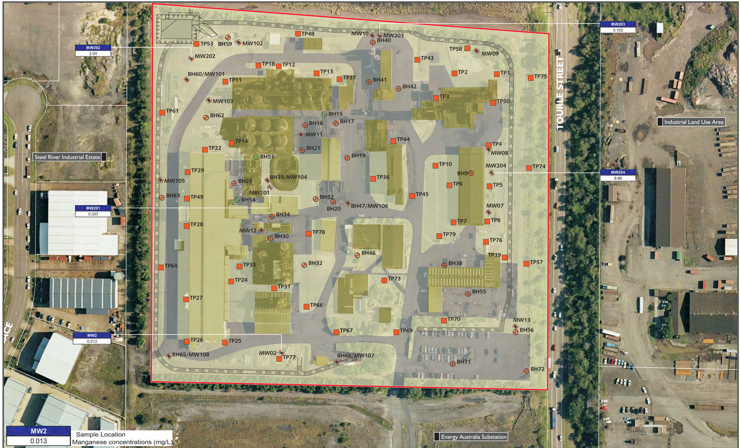
Figure F11 Manganese Concentrations (mg/L) in Deeper Estuarine Aquifer, ENSR 2008 Delta EMD Australia Pty Ltd Data Interpretation and Outline Remediation Strategy McIntosh Drive, Mayfield NSW
