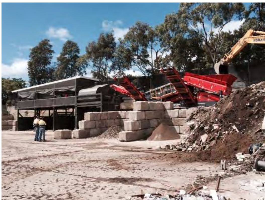
Photograph 2.16 Heavies sorting using a flip flow screen and single picking line
