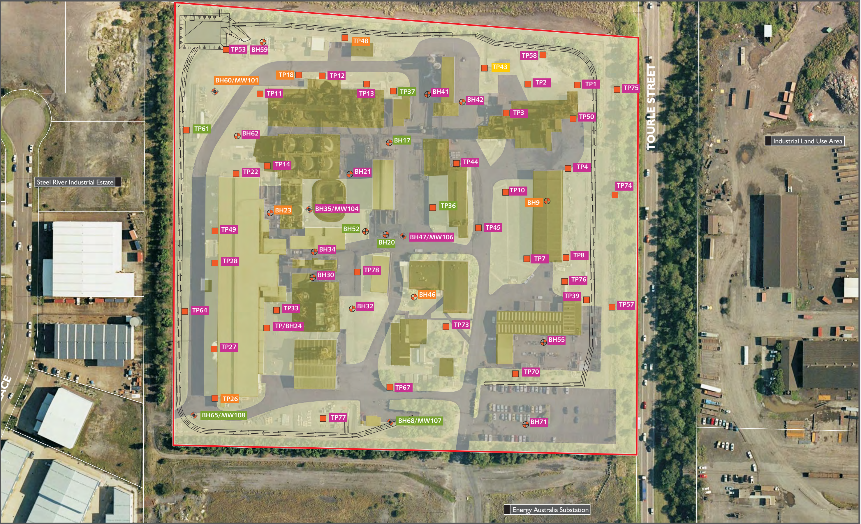
Figure F7 Manganese Concentrations (mg/kg) in Soil (Fill) from 0.5 - 2.0m Depth, ENSR 2008 Delta EMD Australia Pty Ltd Data Interpretation and Outline Remediation Strategy McIntosh Drive, Mayfield NSW
