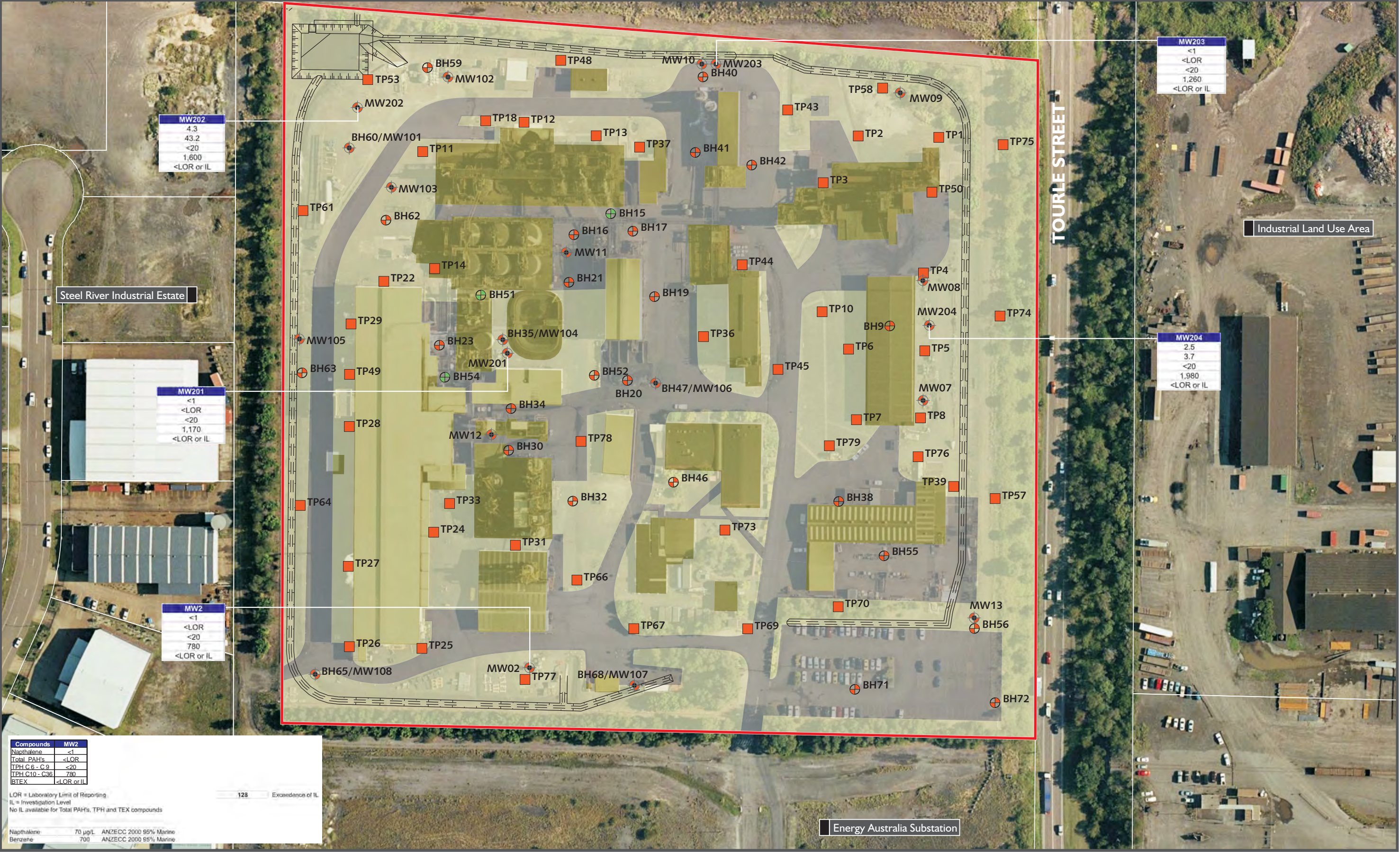
AECOM Figure F13 Organic Compound Concentrations (ug/L) in Deep Estuarine Aquifer, ENSR 2008 Delta EMD Australia Pty Ltd Remedial Strategy McIntosh Drive, Mayfield NSW Note: TP22, TP24 & TP49 were drilled deeper for soil samples and are referred to as BH22, BH24 and BH49 for reporting purposes
