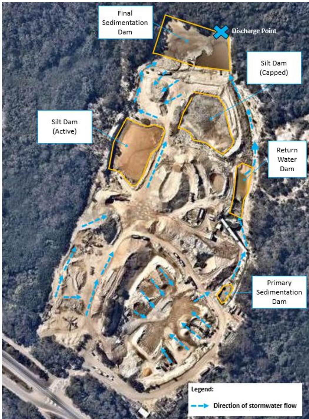
Figure 2a: Site Surface Stormwater Directional Flows
