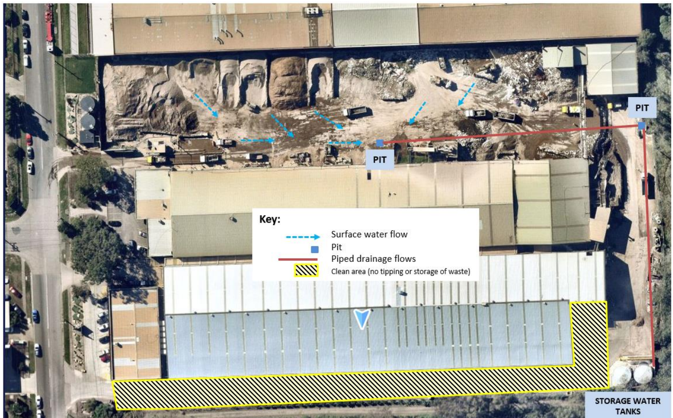
Figure 2: Site Stormwater Directional Flows
