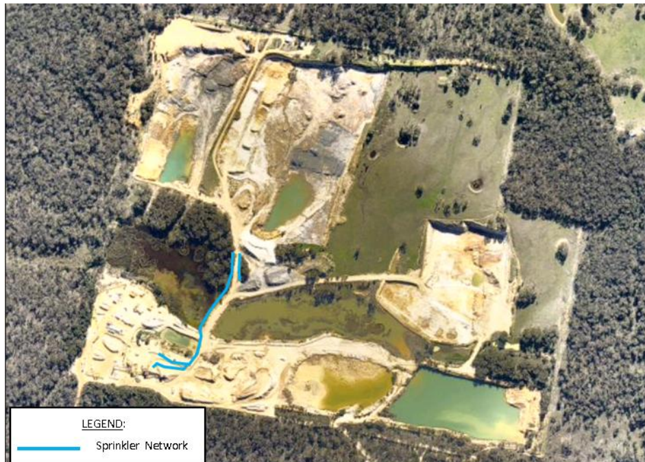
Figure 3 – Dust Suppression Sprinkler Location
