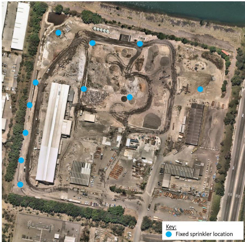
Figure 3 – Dust Suppression Sprinkler Location
