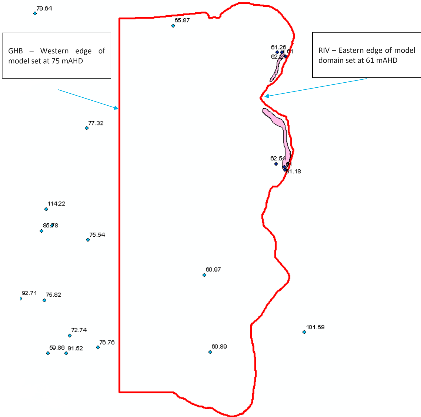
Figure 3.6 Model boundary conditions and regional groundwater levels
